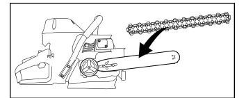
STEP 3 Mount the diamond chain on the guide bar starting at the drive sprocket and continue over the guide bar nose.
